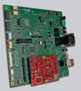
Computer on Modules can be used with standard and custom carrier boards, which host all periphery interfaces, ICs and power control.
